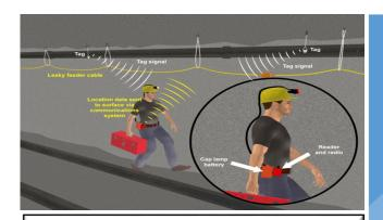
Active RFID 433MHz technology utilizes long range readers and tags that can be calibrated for detection distances less than a meter to hundreds of meters.
