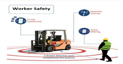
RFID readers and alarms/lights mounted on moving equipment and vehicles and personnel RFID tags are calibrated for safety distances, such as 15' or 100'+. If moving equipment or a vehicle moves into the defined proximity distance of a tagged worker, the alarm and light alerts are triggered on the equipment or within vehicle.
